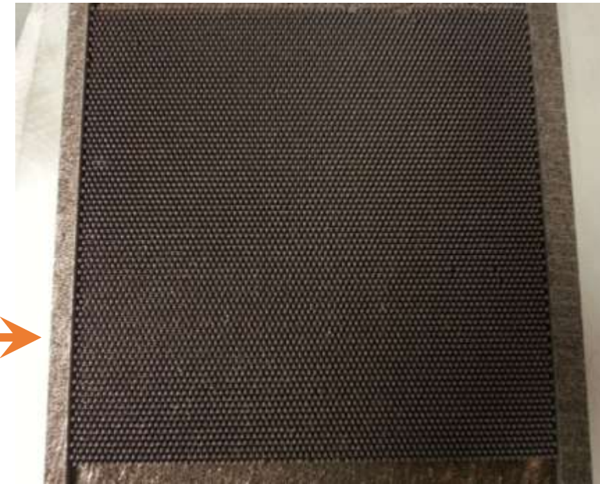
For each layer 6320 elliptical fins
